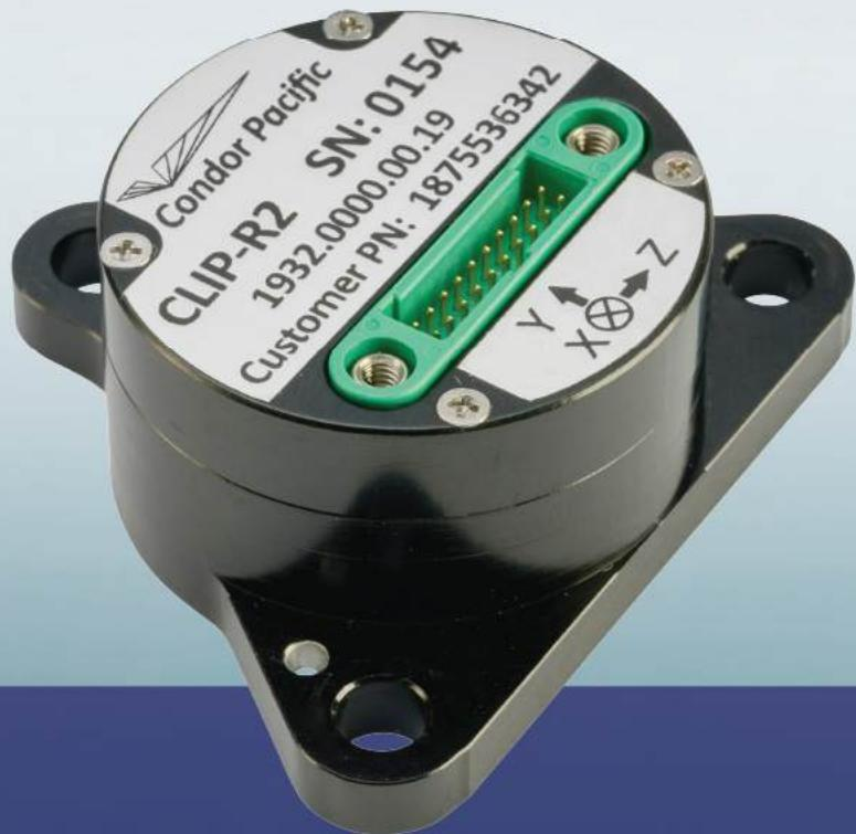
Condor Pacific's CLIP-2 IMU is a field proven versatile MEMS IMU with a configurable digital output. Designed to work under high shocks and vibration, CLIP-2 incorporates 6 MEMS gyroscopes and 6 MEMS accelerometers, all fully isolated and temperature calibrated.
